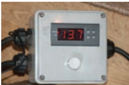
Above: A digital temperature controller, which is used to control the temperature accurately in a warming cabinet.
