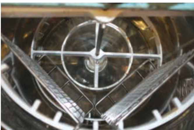
A view looking down into a tangential extractor, where two screens can be seen at the lower edge of the photo.
