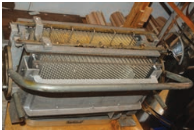
Above: Heather loosener, used to enable frames to be spun using a tangential extractor. All photos on pages 20 and 21 are by Tony Jefferson.
