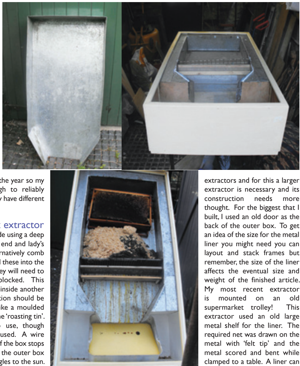
A solar wax extractor deconstructed. Above left: The heat-collecting metal liner made from an old shelf. Above right: The metal liner held in place within an insulating box by wooden spacer pieces. Above centre: Melting wax using solar heat energy: old blackened beeswax has been melted, filtered through three mesh filters and collected in a leak-proof reservoir.
