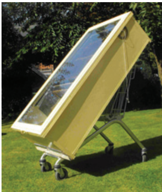
The fully reconstructed solar wax extractor held facing the sun in a supermarket trolley. The solar wax unit, secured tightly so it does not fall when tilted, can be seen through the glazed front. All photos by Dr Chris Coulson.
