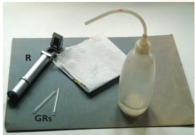
The refractometer kit: the refractometer (R, open), glass rods to apply sample (GRs), distilled or de-ionised water to clean after use (this prevents limestone build-up) and tissue paper. Photo by Chris Deaves.
