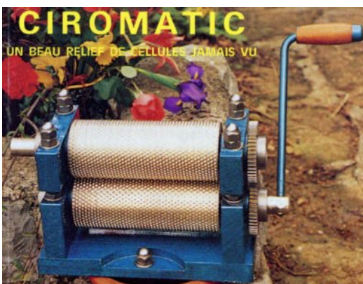
Left: dry embossing with the Ciromatic M.A.T. 37
